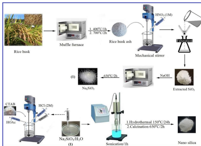
Scheme 1: A cost-effective, energy-efficient and green route for the synthesis of nano silica from rice husk.
